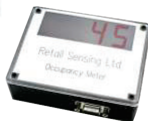
Occupancy meters flash alerts when nearing the maximum capacity
